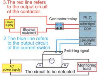
The black line refers to the input circuit of the current switch (the circuit of the equipment to be monitored)
